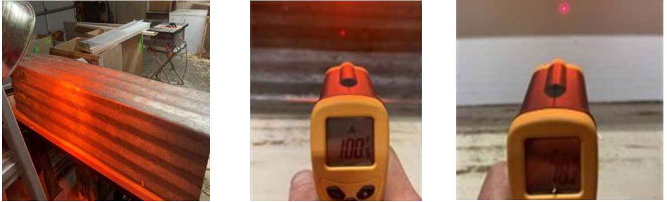
Figure 11: Heat transfer readings of shipping container material.
